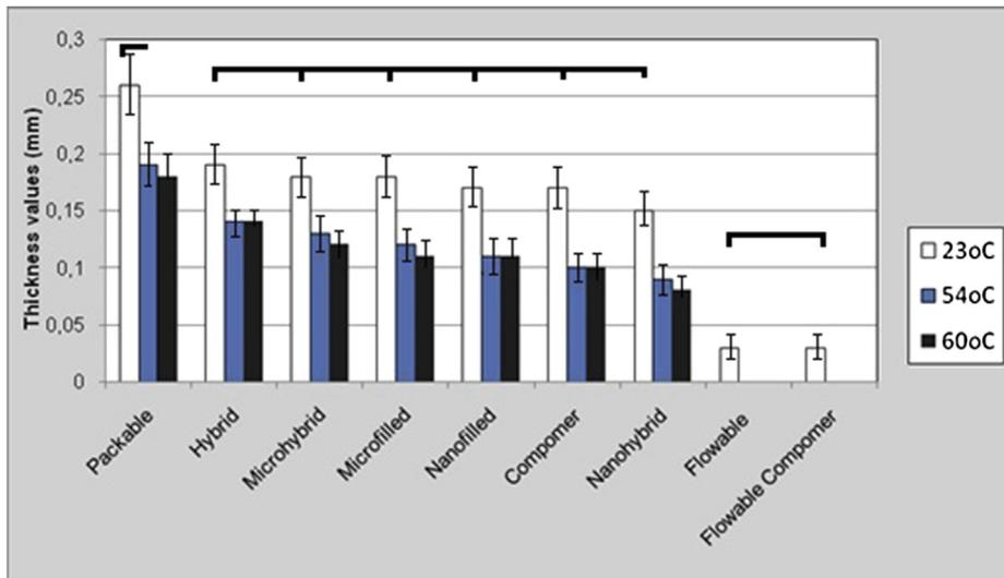
**Figure 3** Mean values and standard deviations of film thickness (mm) of each type of composite material investigated at 23, 54 and 60°C. Horizontal bars indicate no statistically significant differences ( $P < 0.05$ ).
