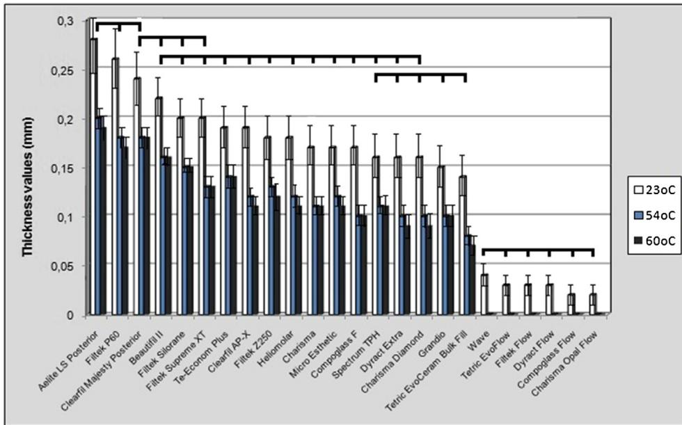
**Figure 2** Mean values and standard deviations of film thickness (mm) of the composite materials investigated at 23, 54 and 60°C. Horizontal bars indicate no statistically significant differences ( $P < 0.05$ ).
