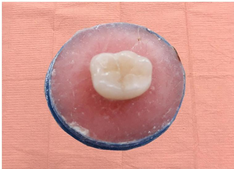
**Figure (2): Tooth mounted in a plastic cylinder using with self-curing acrylic resin**
