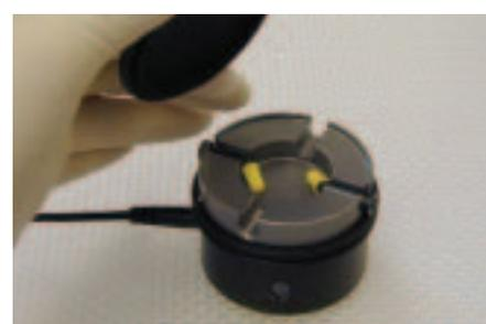
Figure 1—Calset™ heating unit with compules in place.
