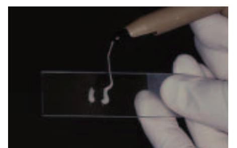
Figure 3—When heated to 130°F, the material takes on a honeylike consistency.
