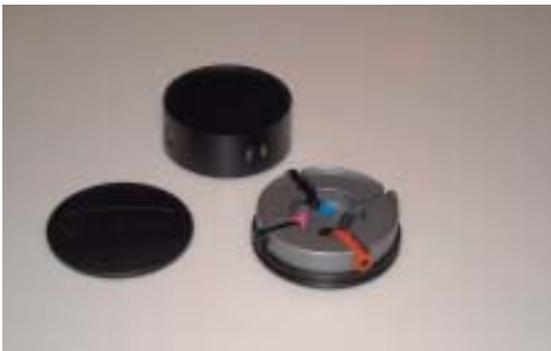
**Figure 9**—The top segment of the Calset can be removed and transported independently.
