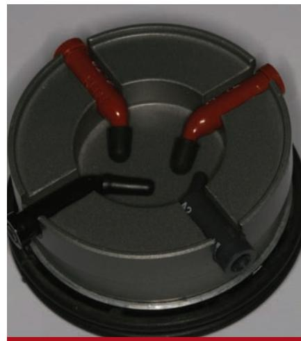
**Figure 12** The CalSet veneer warming tray is preheated to 155°F.
