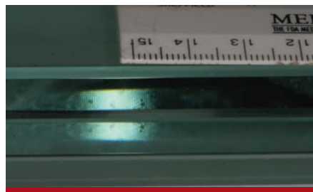
Figure 1 Each composite resin was placed between two glass slabs at room temperature.
